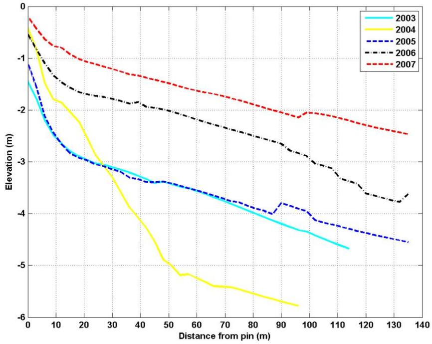
**Figure 134.** Mean annual profiles for WE1 showed stability between 2003-2005; it is difficult to gauge profile changes since the starting point changed between 2005-2006. Accretion occurred between 2006-2007.
