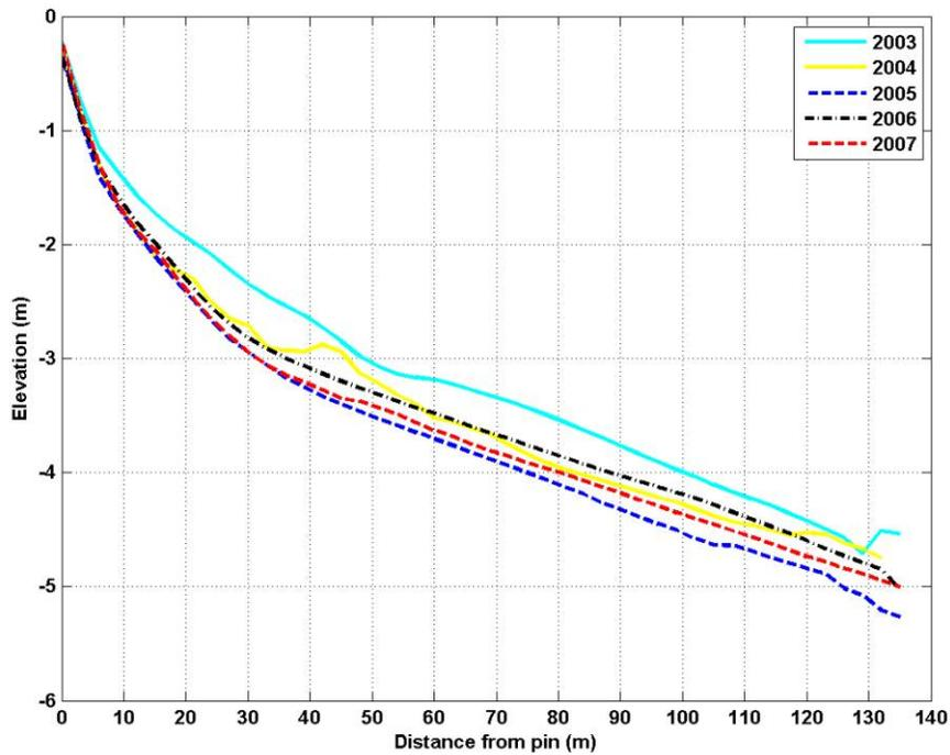
**Figure 137.** Mean annual profiles from WE2 show that the beach underwent erosion from 2003-2005, then recovery in 2006, and additional erosion in 2007.
