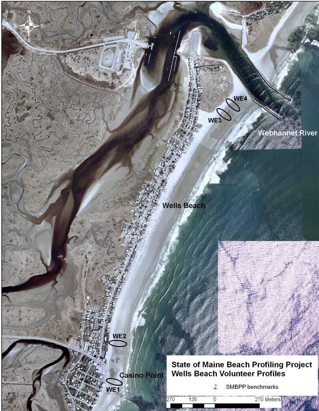
**Figure 133.** Wells Beach has 4 measured beach profiles, WE1-WE4. The starting marks for the profiles have not been surveyed by MGS as of April 2007. The 4 profiles are approximately located on the figure.
